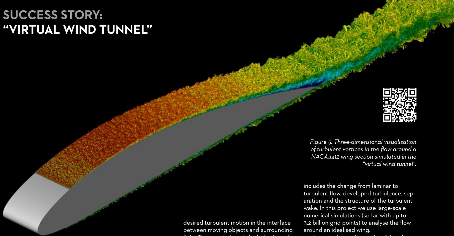
Figure 5. Three-dimensional visualisation of turbulent vortices in the flow around a NACA4412 wing section simulated in the “virtual wind tunnel”.
